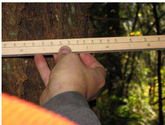
Figure 6-2: To measure DBH with a woodland stick, hold the stick against the tree at breast height, 25 inches from your eye. Keeping the stick level and perpendicular to your line of sight, line the end up visually with the left side of the tree. Then move your eyes (not your head) to read diameter on the right side of the tree. In this case, the tree whose DBH measured 34.0 inches with the diameter tape in Figure 6-1 measures between 33 and 34 inches with the woodland stick.
