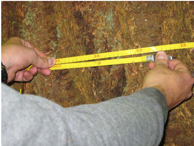
Figure 6-1: To measure DBH, wrap a diameter tape around the tree at breast height, making sure the tape is level and not twisted. The diameter measurement is read where the tape overlaps with the zero marker. In this case, the DBH of this tree is 34.0 inches.
