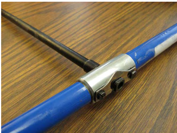
Figure 6-11: An increment borer is assembled by inserting the back end of the bit into a notch in the center of the handle and clipping into place.
